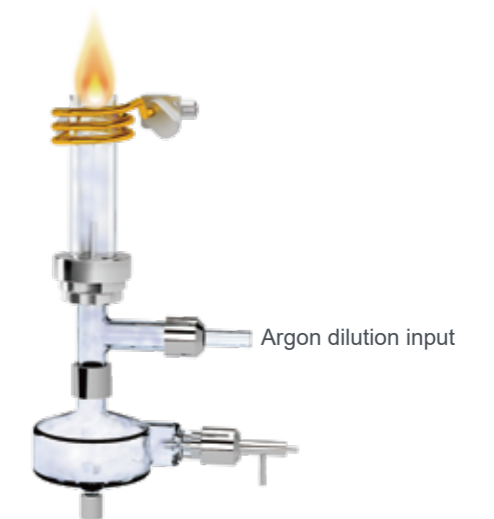
Schematic diagram for argon dilution input
