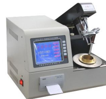
Closed flash point tester
